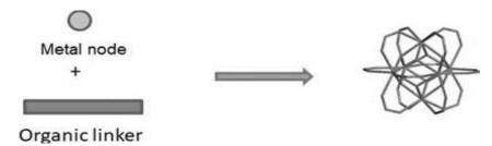
Fig. - 1: Direct assembly of MOFs from metal node and organic linker
