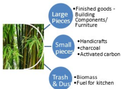
Figure - Main and by-products of bamboo processing
