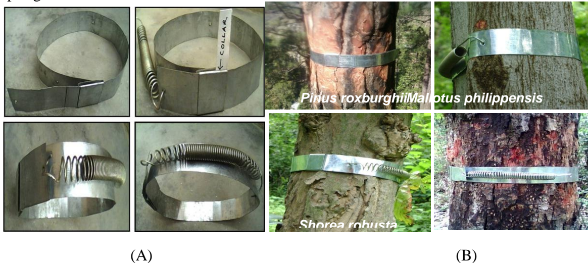
Figure 2: (A) showing dendrometer bands and (B) dendrometer bands tied over the trees.
