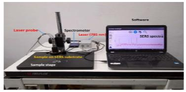
Portable Raman set-up under developing stage in lab. Trials are running on the system to optimize. Miniaturization in the form of hand-held device is to be done.
